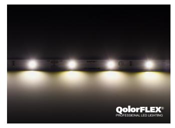
**QolorFLEX LED Tape, Warm White, 12V Indoor (P/N 3528-12-WW-30-5-20-1)** is an interior grade LED tape with a medium low output (150 lumens/metre) brightness in a warm 2700°K colour temperature. Each LED tape comes with wiring leads on both ends and durable 3M adhesive backing. It is available in full five metre reels and sample strips.
